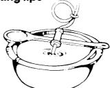
For liquids, balance the probe on a wooden spoon or spatula so the tip of the probe is in the center of the liquid.
